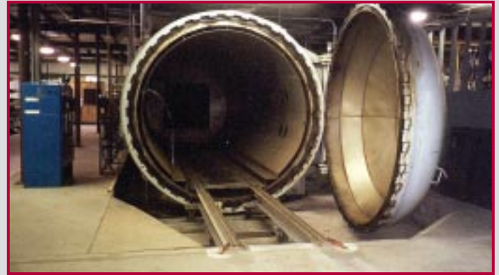
MELCO 25' AUTOCLAVE (FRONT VIEW)
